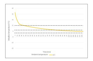
Heating performance at ambient temperature Model S Cool
