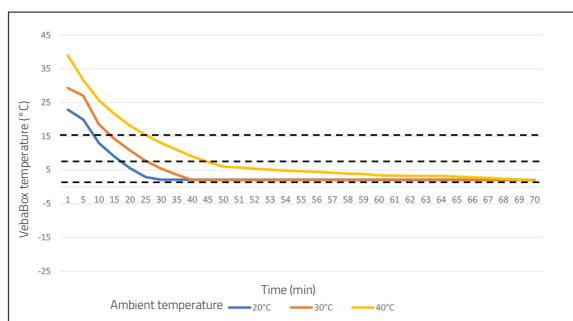
Heating performance at ambient temperature Model M Cool
